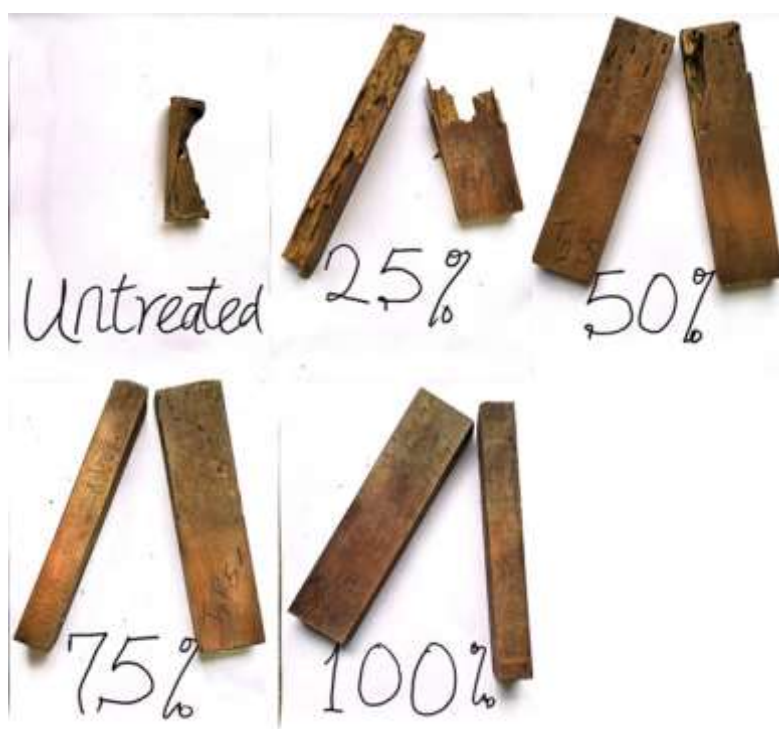
Fig. 5. Wood samples of untreated (control) and treated Alstonia boonei after exposure to termite attack.
